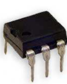
Fig. 5.5.4 Using a MOSFET Relay chip for switching A.C. or D.C.
