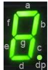
Fig. 2.4.5 LED 7 Segment Display
