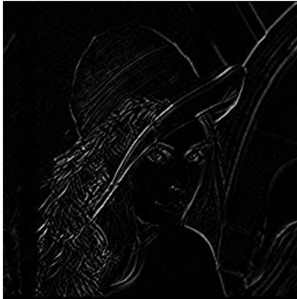
Figure 2.2.24 Result of the line detect operation on LENNA.
