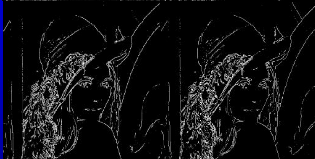
Output of the one-pass thinning algorithm
