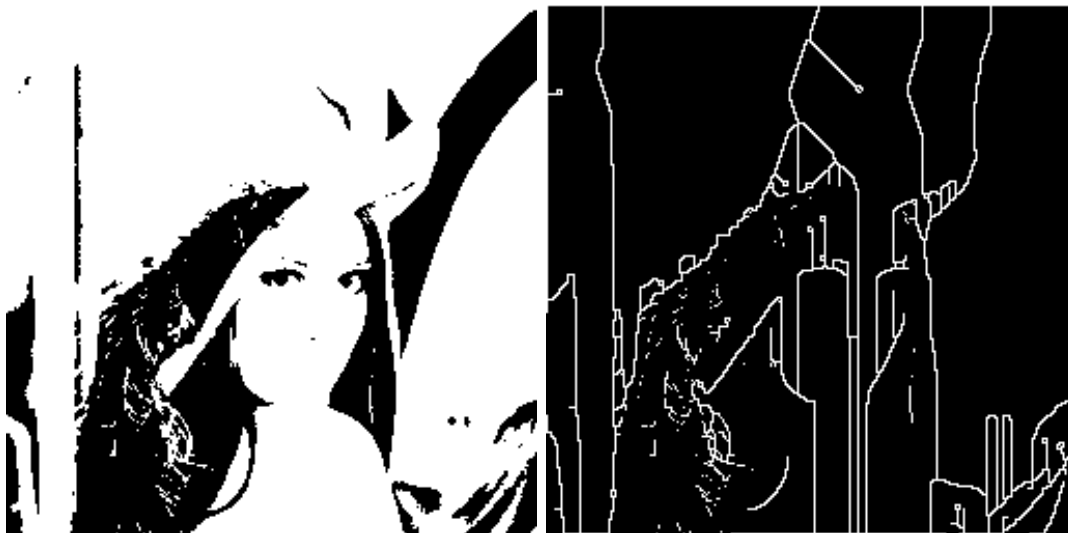
Figure 2.2.31 Thresholded LENNA and the result of one-pass thinning.
