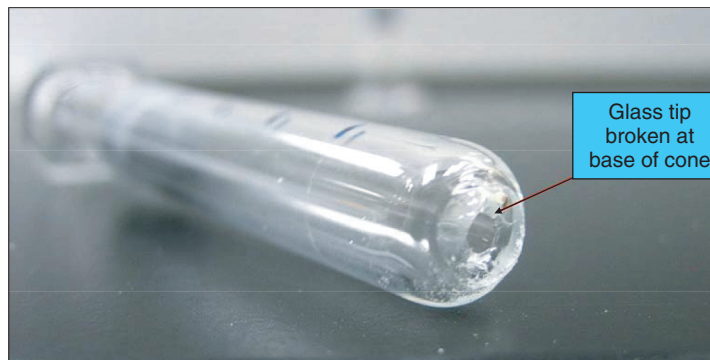
Figure 36.8. A 1-mL-long syringe barrel after breaking off the tip at the shoulder. The resulting hole in the barrel is large enough that product fluid flow resistance is no longer a factor when measuring glide force.
