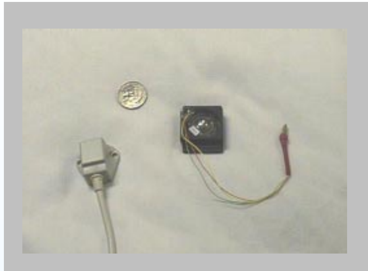
Fig. 2. The electromagnetic sensor (left, Ascension Technology) and the tilt sensor (right, Microstrain). A quarter is shown for size comparison.
