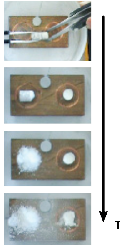
Figure 7.7. Amorphous ice sample (1.5 mL) made by decompression of VHDA (see Section VII) at 140K to 0.07 GPa with a rate of 13 \text{ MPa min}^{-1} and then quench-recovered to 77K and 1 bar (top image). After removal from the piston cylinder apparatus, the sample easily broke into two pieces; the two separated pieces were placed on a copper block kept at 77K (second from top). The bottom two images show the two pieces in the course of heating to 250K at 1 bar. Adapted from Ref. [68].
