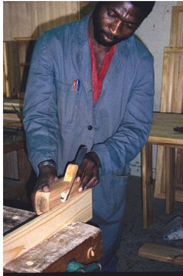
Figure 1 : Tool-making training in Zimbabwe. Mr. Buekerwa tests a rebate plane. Photo: Aaron More / Practical Action 1991.
