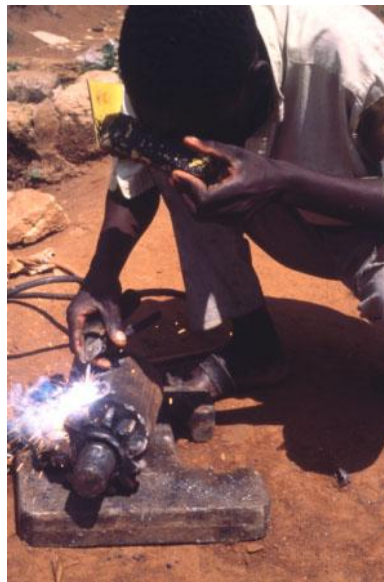
Figure 1: Kennedy Otieno repairing a sugar crusher for jaggery production. Migori, Kenya Photo credit: Practical Action/Morris Keyonzo
