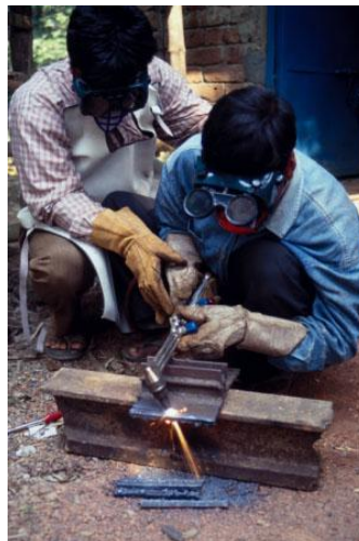
Figure 4: Flame cutting. Practical Action organised training for Asaduzzman Munshi in welding. As a result he has now started a small metal workshop of his own, earning Tk 3000 monthly (2000). In the process of cutting parts for a three-wheel rickshaw structure. Photo credit: Practical Action/Zul
