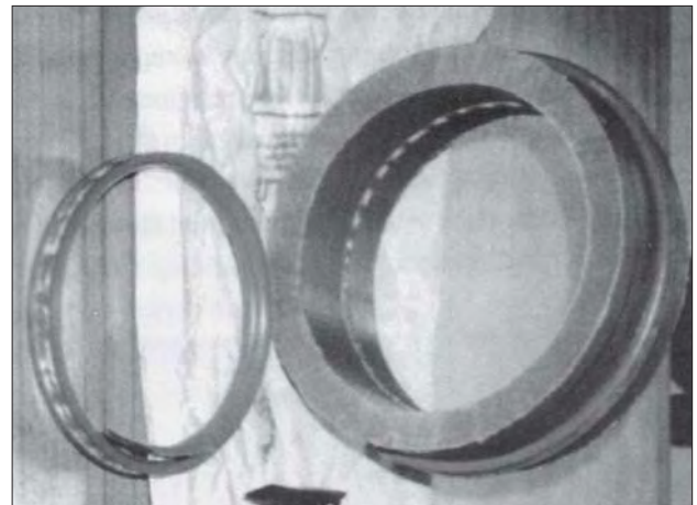
Photo10.5 HDPE pipe joint de-beaded using a commercial de-beader. The small ring in front of the pipe section is the bead.
