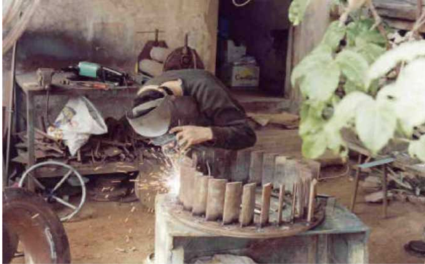
Figure 15: Positioning of the guide blades
