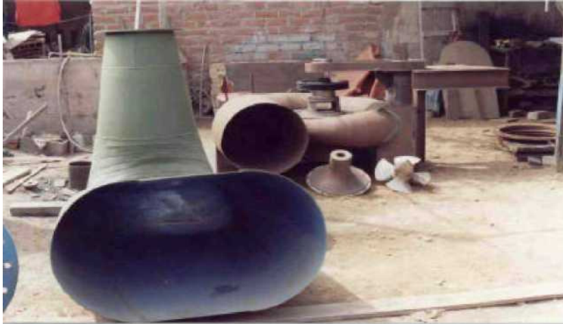
Figure 3: Suction tube manufactured from sheet steel
