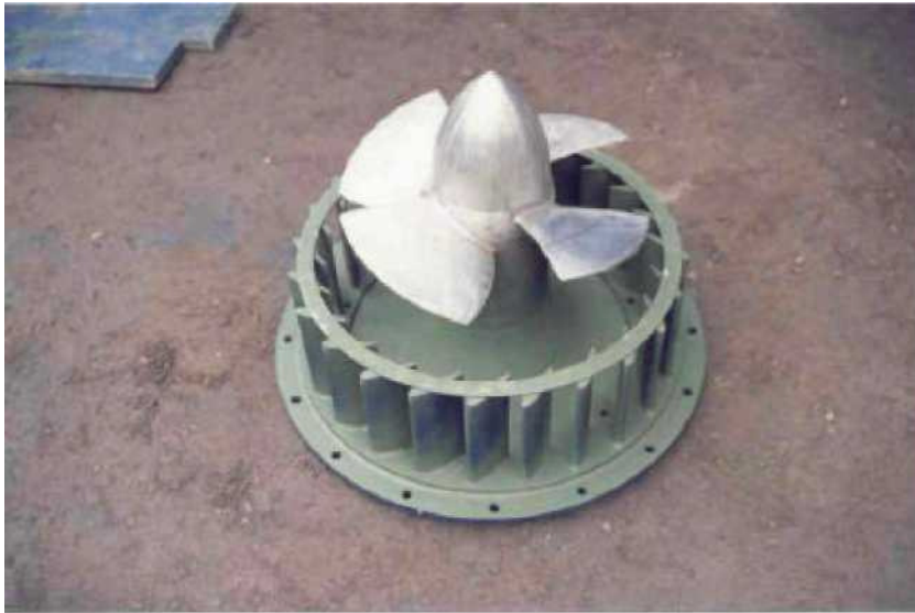
Figure 1: Stainless steel wheel mounted on guide blades
