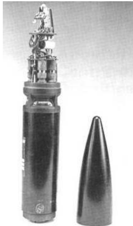
Fig 19.3 EMI proximity Fuse in the nose of a 3.7 inch anti-aircraft shell with the nose cone removed to show the electronics.
