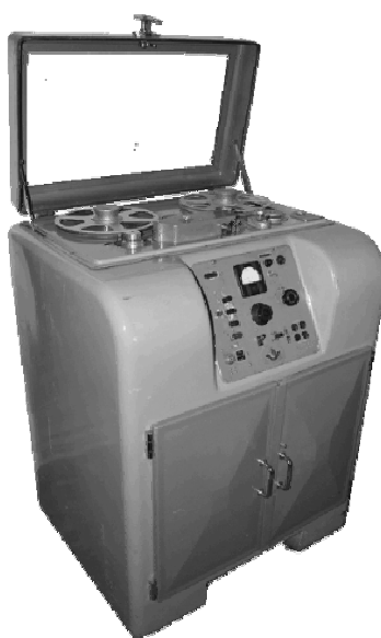
Fig 20.3 BTR1 Studio tape recorder
