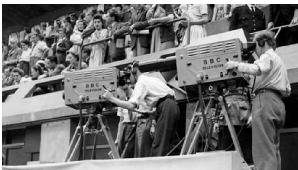
Fig 20.1 CPS Emitron Cameras in use at the Wembley Empire Pool for the 1948 Olympic Games
