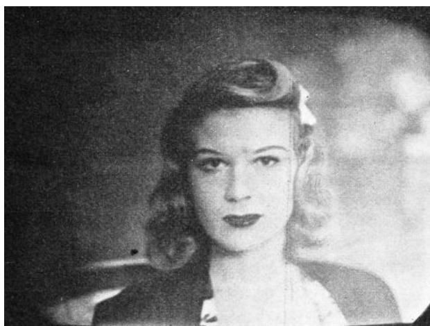
Fig 14.2 An uncorrected Emitron image showing the secondary electron shading.
