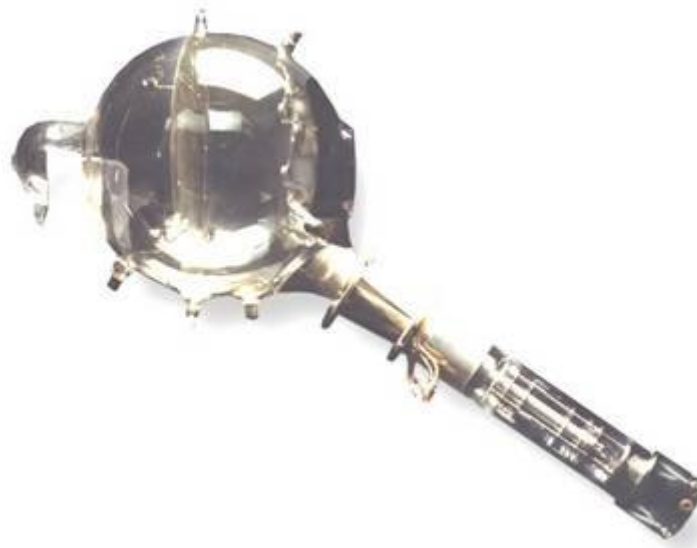
Fig 13.2 An early Emitron camera tube. The long stem on the right contains the electron gun with its focusing electrodes and deflection coils and the optical window is above it. Inside the sphere is the mosaic. The ‘tail’ on the left is where the tube was sealed.
