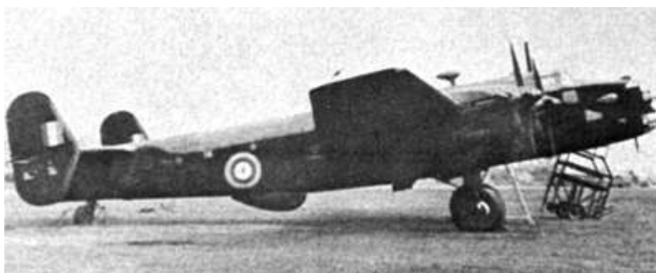
Fig 18.2 The Halifax bomber with the prototype H2S system before the crash. The radome with the scanner can be seen under the roundel towards the rear.
