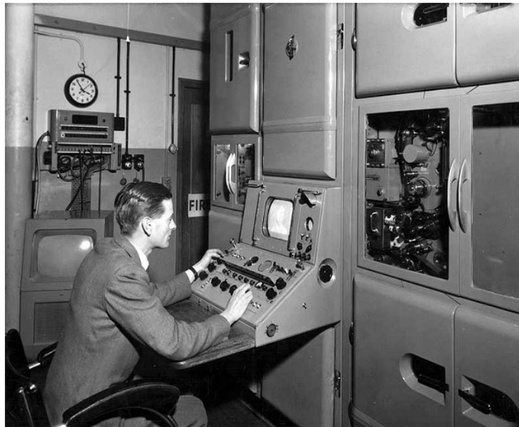
Fig 20.2 EMI Flying Spot telecine system. On the right of the operator is the 35 mm film section and the left the 16mm.
