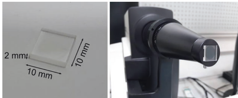
Fig. 18.16 Photograph of phase plate (left image), and the photograph of SPECTRALIS with phase plate (right image)
