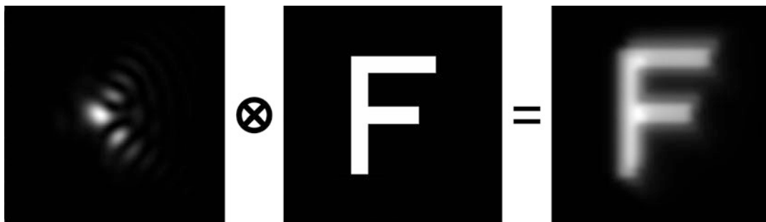
Fig. 18.4 Image formation process. The final image generated by the optical system can be described as a mathematical convolution of the object with the PSF of the optical system
