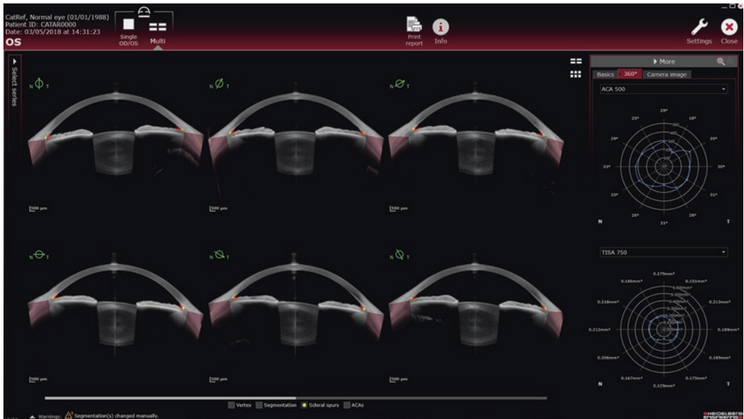
Fig. 13.18 ANTERION Metrics App multiview. OCT images of the whole anterior chamber and 360° ACA 500 and TISA 750 graph analysis
