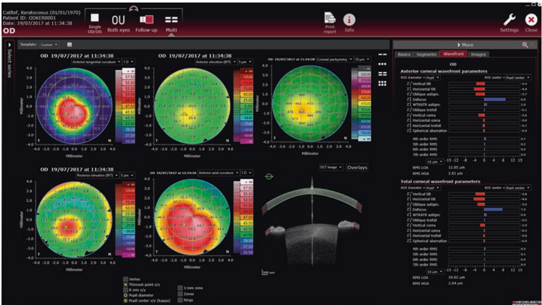
Fig. 13.9 ANTERION Cornea App multiview. Five corneal maps (anterior tangential curvature, anterior elevation, corneal pachymetry, posterior elevation and anterior axial curvature), OCT image and wavefront parameters of a keratoconus eye
