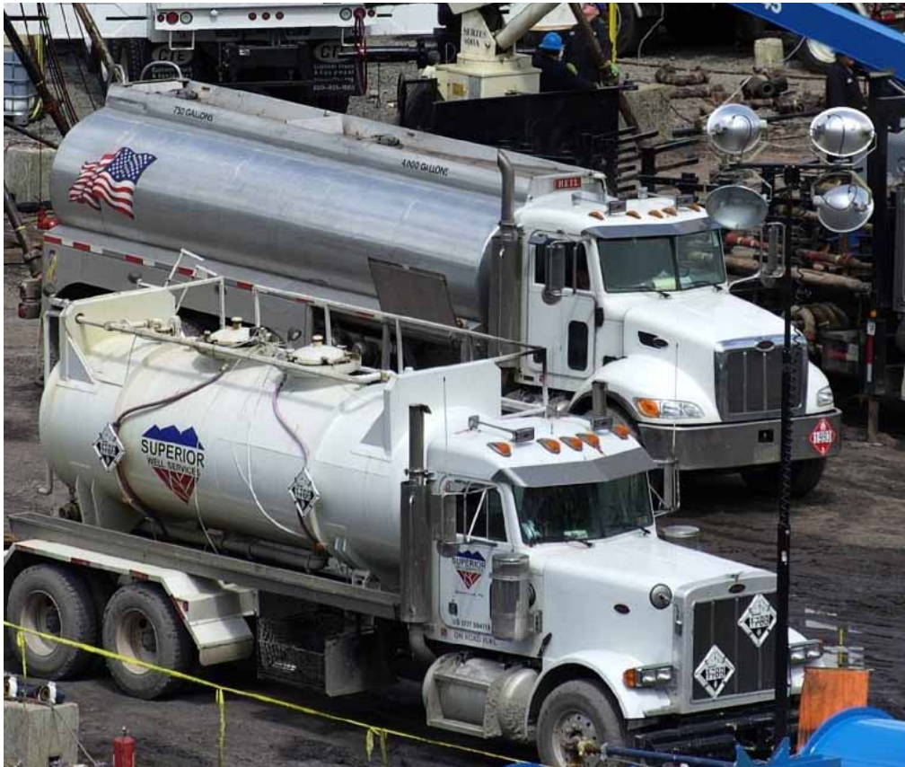
Trucks delivering fracturing water (above) and hydrochloric acid (below) to a well site.
