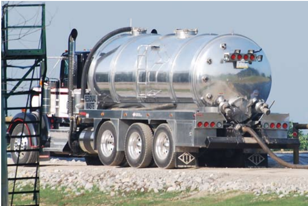
A tanker truck loading fracturing wastewater from a storage pit for disposal at a sewage plant.
