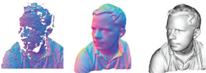
Figure 1: Example output from our system, generated in real-time with a handheld Kinect depth camera and no other sensing infrastructure. Normal maps (colour) and Phong-shaded renderings (greyscale) from our dense reconstruction system are shown. On the left for comparison is an example of the live, incomplete, and noisy data from the Kinect sensor (used as input to our system).
