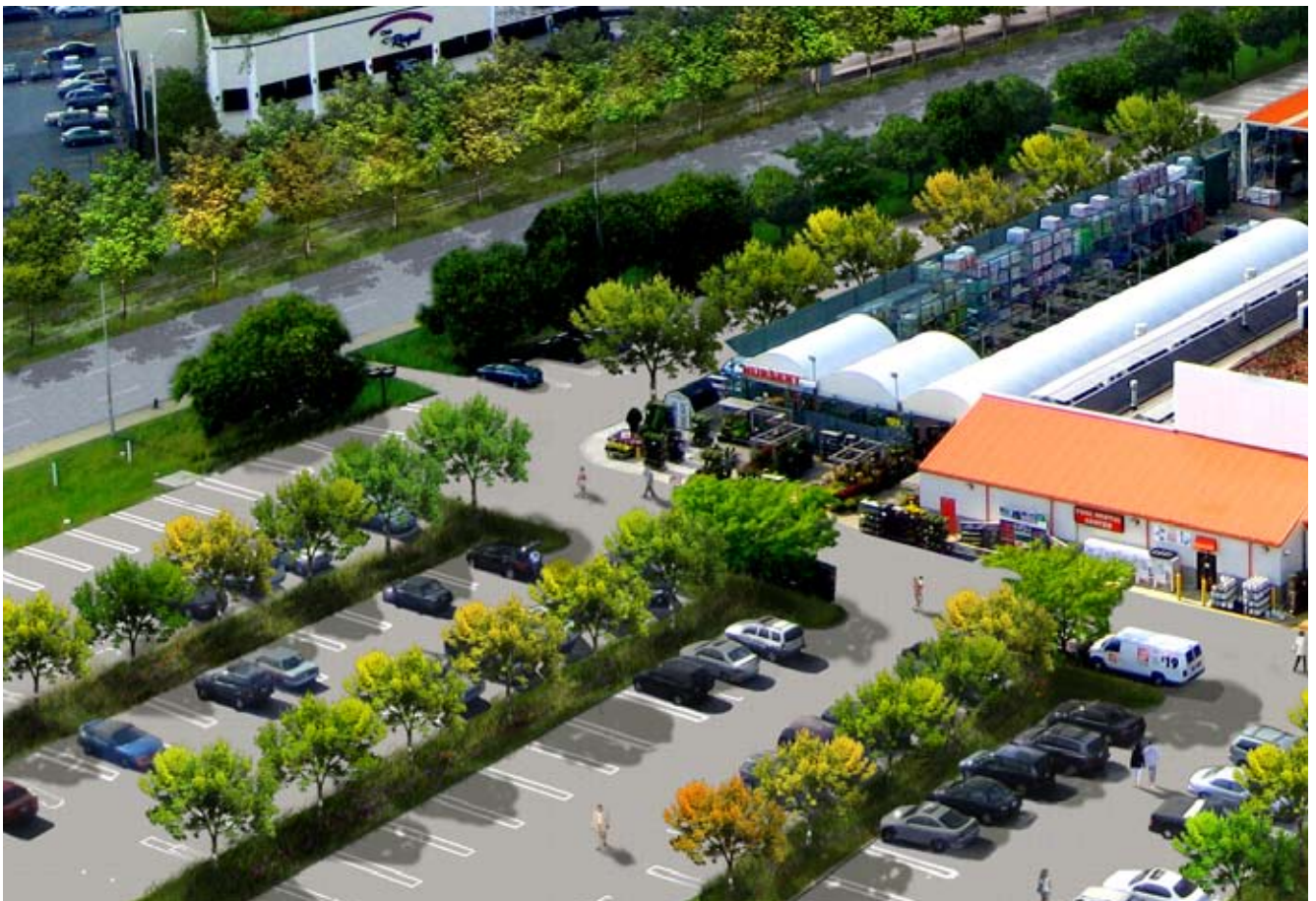
Above: A vegetated swale collects and infiltrates stormwater from an employee parking lot at the Philadelphia International Airport in the Schuylkill Watershed.
