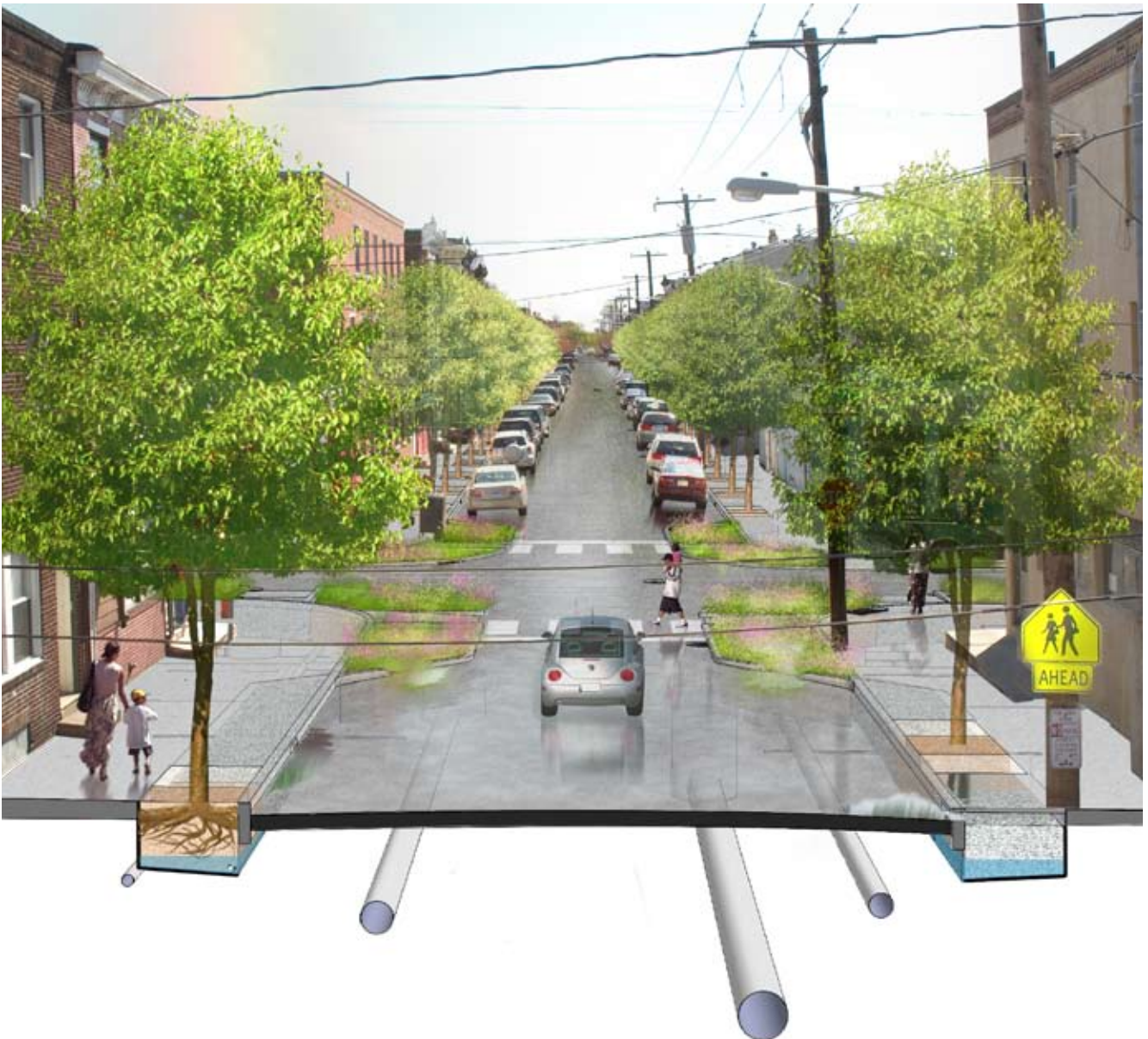
Above: Street runoff is captured at this rain garden at 47th St. and Gray's Ferry Ave. in the Combined Sewer Area within the Schuylkill River Watershed.
