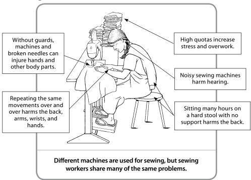
Machine injury: Needles in the machine can cut your fingers and hands and can break and fly into your eyes. Moving parts can catch hair and pull it out or pull a person into the machine.
