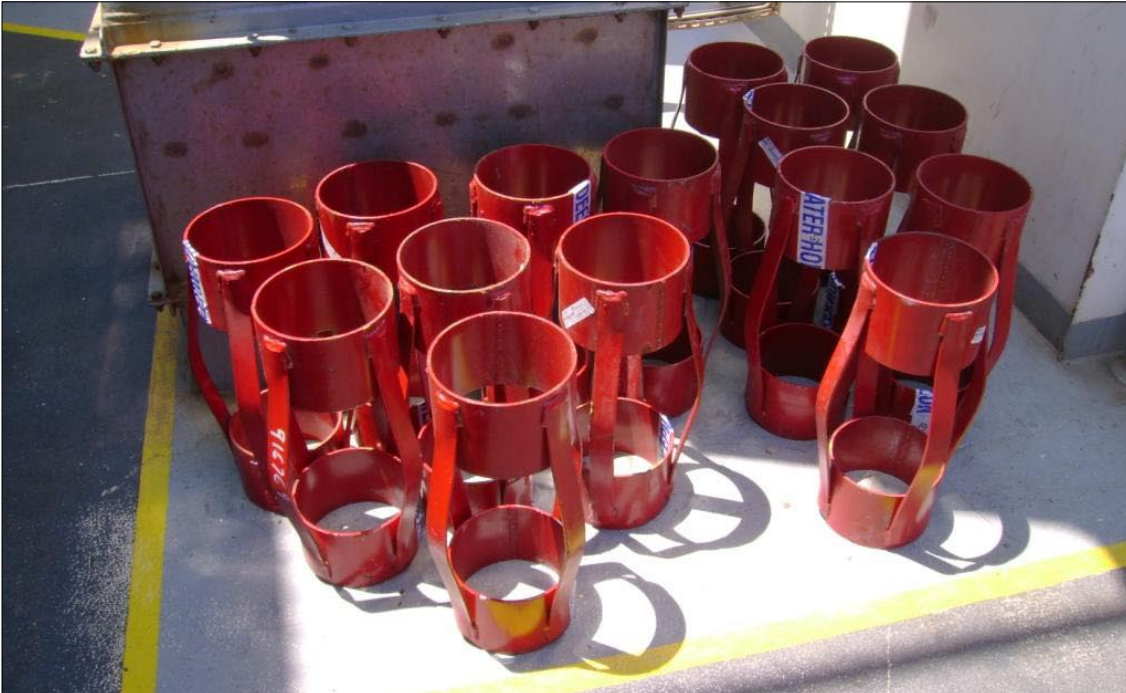
Figure 4.3.15. Centralizers delivered to the Deepwater Horizon on April 16, 2010.
