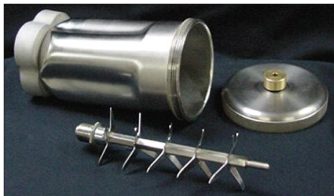
Figure 4.4.1. Foam testing apparatus.
