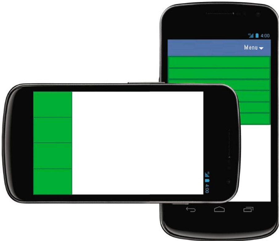
Fig. 6. Application navigation bar adaptation for mobile and tablet devices based on screen orientation
