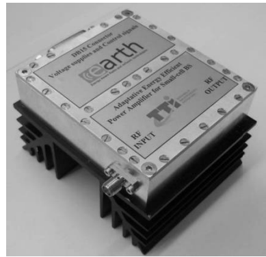
(b) Adaptive power amplifier
