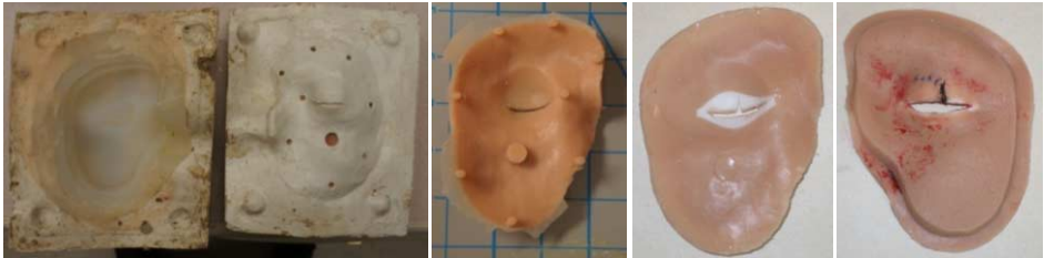
Figure 4: Molding of eye portal - production mold, early single material eyelid models; eye lids with "tarsal plates" (back and front after suturing during data collection scenario).
