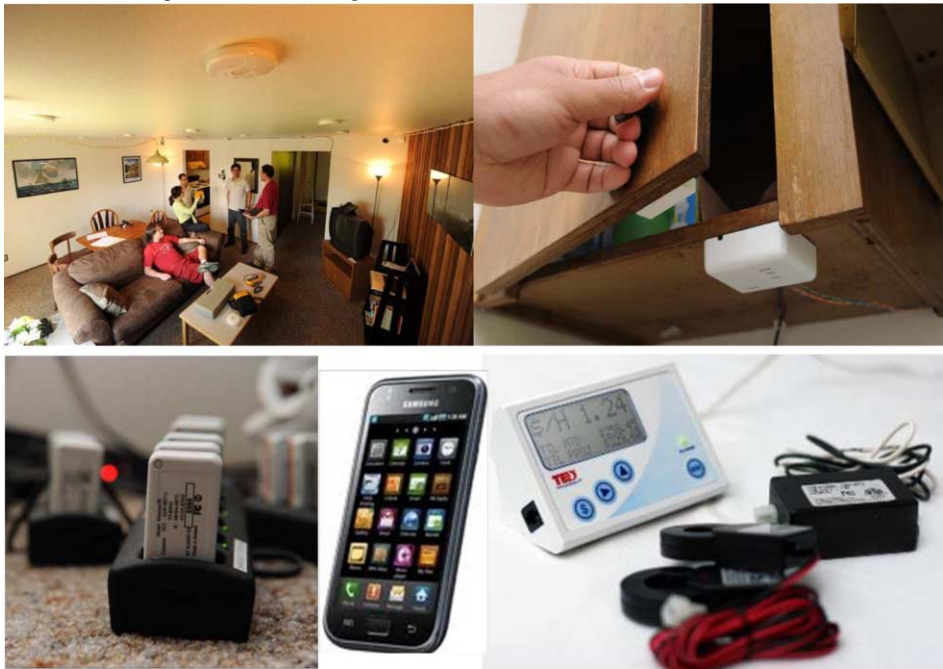
Figure 3.3. CASAS in A Box sensor components, including motion / lighting sensors attached to the ceiling (upper left), door / temperature sensors (upper right), object shake sensors (lower left), smart phone (lower middle), and TED power meter (lower right).
