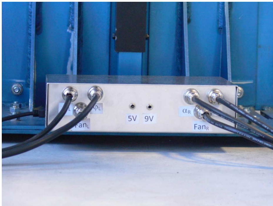
Figure 2 The embedded electronic board and its connection with the sensor on the platform
