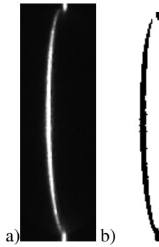
Figure 3. Segmented line by the Otsu method. a) Original image and b) Segmented image.
