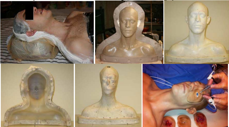
Figure 3: Molding sequence for prototype head-form. Life casting. Clay duplicate. Plastic positive with 3D scanning fiducial marks. Silicone production mold. Plaster core with 3D scanning fiducial marks, air holes for skin casting. Final molded silicone skin, with pigmentation and replaceable trauma modules.
