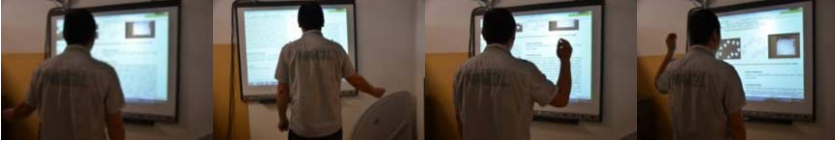
Figure 4 Gesture Interact of user in IZ (scroll up, down, zoom in and out)
