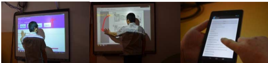
Figure 1 Proxemic Platform (Left: hand cursor control, Middle: scroll by hand glide, Right: file migrator)
