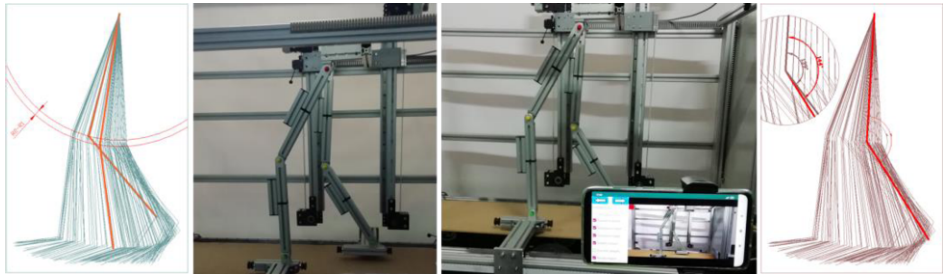
Figure 6. Test C. Left: selected angle measurements from human captured swing stage. Centre: Rig walks. Right: visualization and measurements on selected frames.
