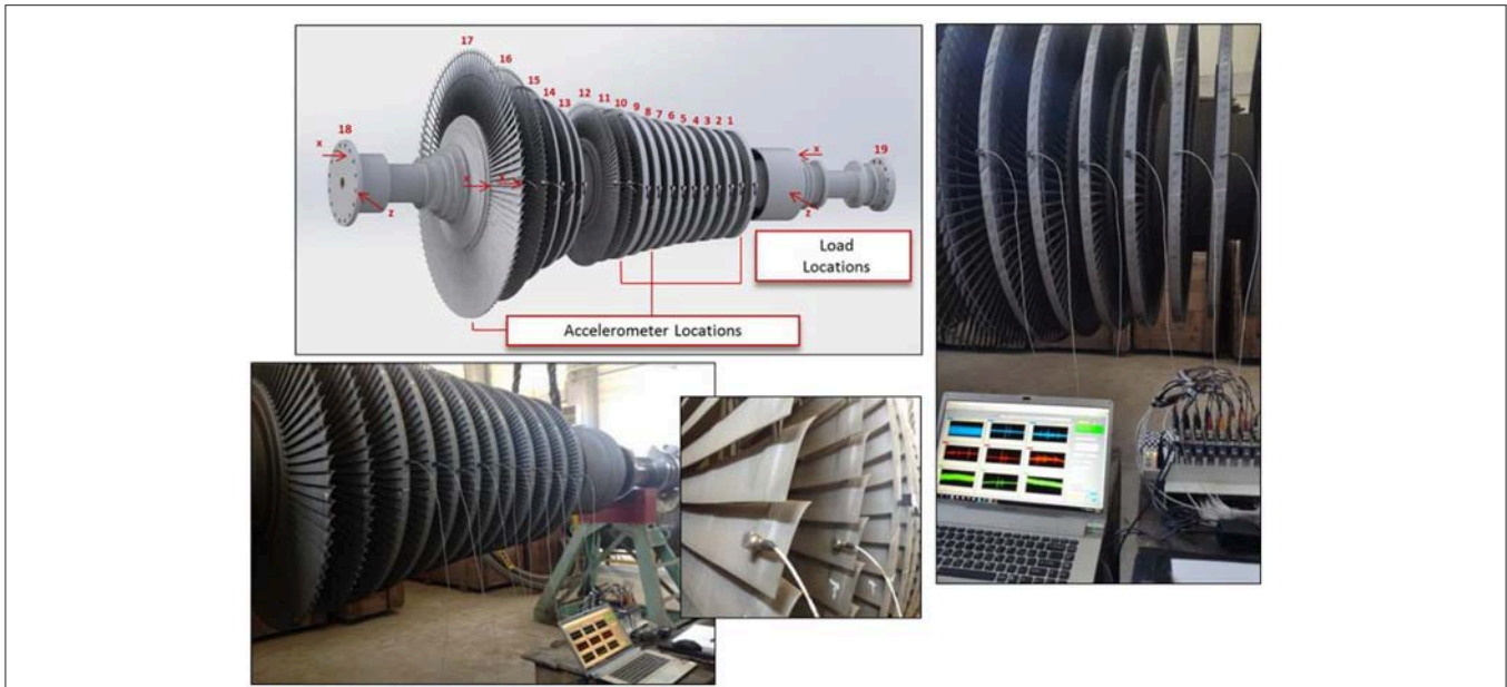
FIGURE 7 | Experimental set-up of the intermediate pressure turbine.
