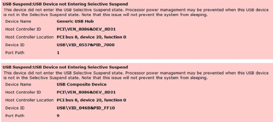
*Figure 7-10. A portion of the energy report generated by the Windows Powercfg tool*
