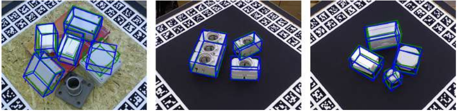
Fig. 4. Qualitative pose estimation results on T-LESS. The blue boxes indicate estimated poses and the green boxes indicate ground truth poses. (Color figure online)
