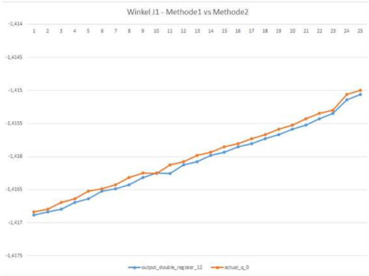
Fig. 4. Latency-Measurement in 8 ms steps. Status values directly from RTDE (actual_q_0) and values read from URScript and transferred via RTDE (output_double_register).
