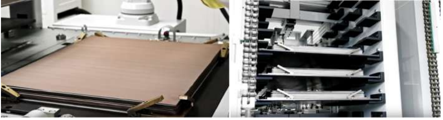
Fig. 4. PCB fabrication: lamination and curing cycle. Pre-assembled stack-up (left) and 20 positions loader of a Lauffer press. (Courtesy of Somacis, Italy)
