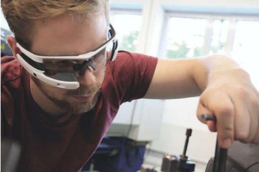
Fig. 1. Smart glasses as part of industrial live video assistance systems
