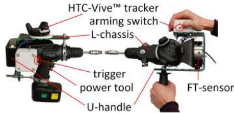
Fig. 2. Hardware setup of the Instrumented Tool, including tracking and force/torque sensors [19].
