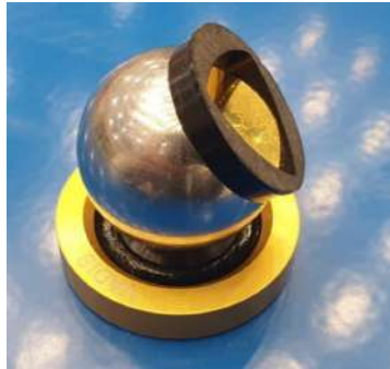
Fig. 15. Jig reference system nest and ID ring with SMR
