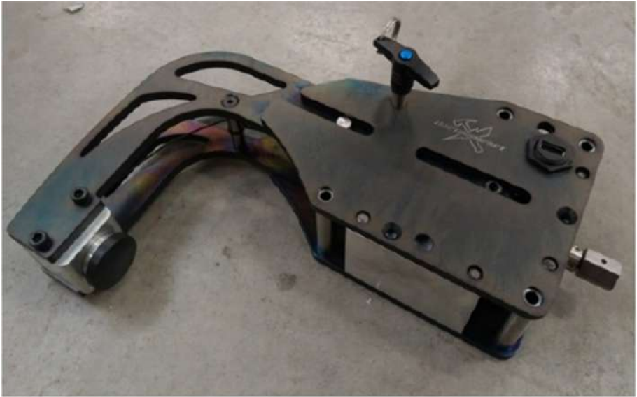
Fig. 17. Manual panel clamp with load cell feedback
