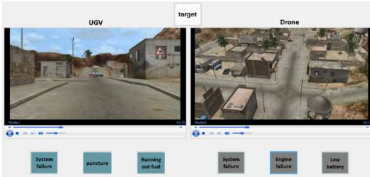
Fig. 2. The visual display where participants received the alerts and responded to them (touchscreen, screen #3). On the top is the target indicator and on the bottom are the various failures that could have occurred for the UGV and drone.
