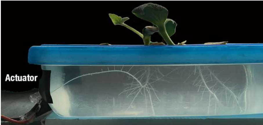
Fig. 1. A prototype with an Arduino Uno driving a Tectonic Elements TEAX25C05-8 transducer with a 250 Hz sine wave. The image shows results of approximately two weeks of continuous stimulation on the root orientation of pumpkin seeds ( Cucurbita maxima ). One root can be observed to orient towards the source of vibration. Root growth would be expected to be more diffuse without stimulation, though, note, this is a single-trial result for illustration purposes.
