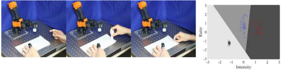
Fig. 2. (Left) Human states recognized by the SVM: no contact, gluing, tracing. (Right) Example of SVM model where data are well separated considering the intensity and ratio parameters (black: no contact, blue: gluing, red: tracing). (Color figure online)
