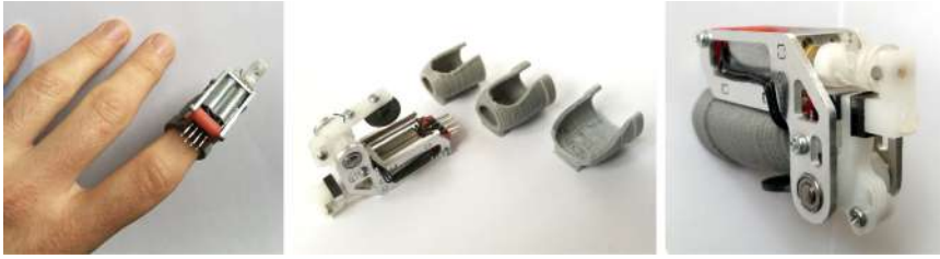
Fig. 3. The slim lateral profile of the device (left) allows easy switch of rubber thimbles with different finger sizes through a slider mechanism (right)
