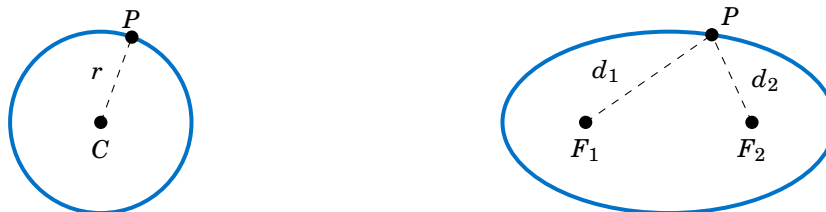
(a) Circle: center C , radius r = \text{constant} (b) Ellipse: foci F_1 and F_2 , d_1 + d_2 = \text{constant}
