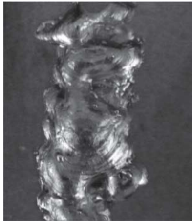
Figure 2. Laboratory sample of NOK weld.
