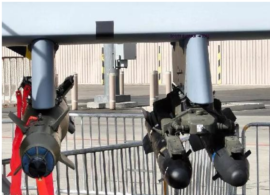
Figure 11-4 Typical Reaper Load Out with the Hellfire Missiles on the right and a GBU-12 on the Left
