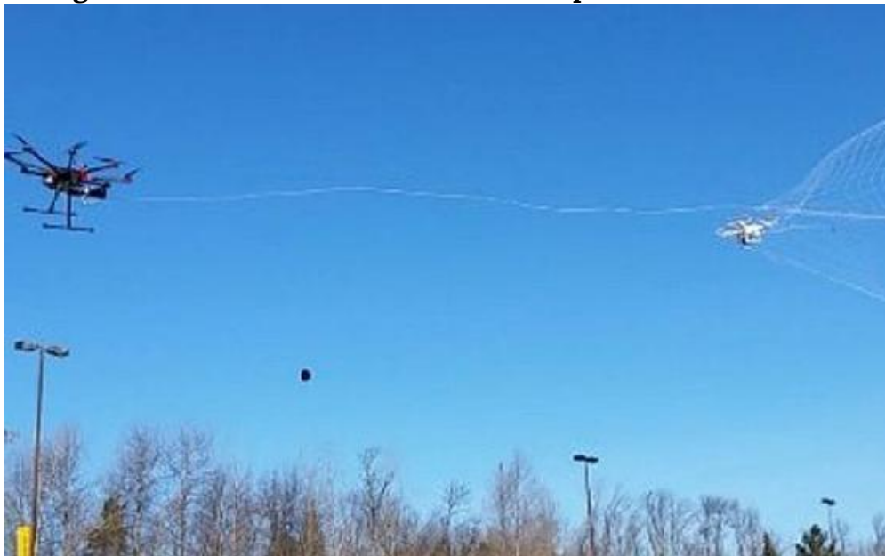
Figure 11-14 Drone launches a net to capture another drone
