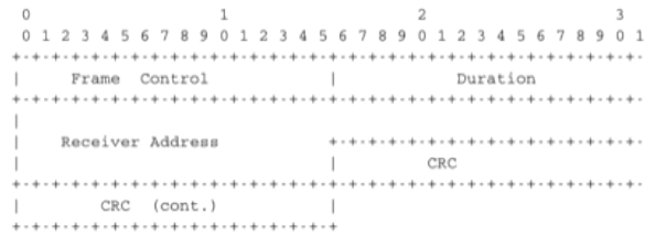
Figure 6.35: IEEE 802.11 ACK and CTS frames
