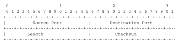
Figure 4.35: UDP Header Format
