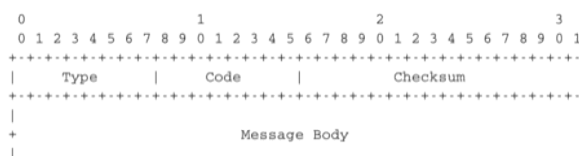
Figure 5.42: ICMP version 6 packet format
